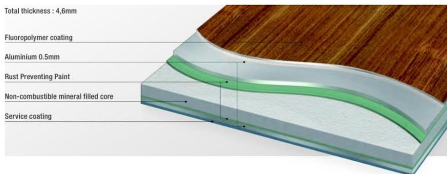
It is important to understand that "fire retardant" ACM's are constructed using a wide variety of materials and methods and as a result they do not all perform in the same way in relation to fire. To assist identification of fit-for-purpose ACM cladding, the current CodeMark Certificates disclose their non-combustible component. This is a major advancement in the area of transparency as all material components will be assessed independently and without embellishment.
